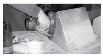
Step 3: Cut insulation to fit the base of the plywood box and the four sides (See picture below). Place the aluminium box inside the plywood box with the insulation between the two. The fit should be snug. Newspaper could be used in place of insulation, either scrunched up in balls or torn into shreds then packed first on the base and then between the walls of the two boxes.
