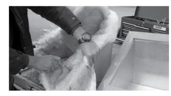
**Step 4:** With the insulation firmly in place, join the plywood oven top to the outside case using glue and small nails evenly separated.
