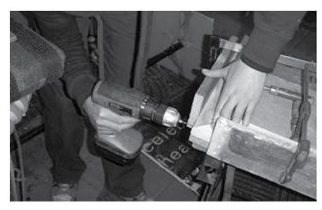
**Step 3:** Unclamp the two pieces of wood and apply wood glue. Re-clamp and drill a screw into the pre-drilled hole.
