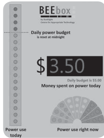
The concept design for the BEEbox (Bushlight Energy Efficiency box) in-home display.
