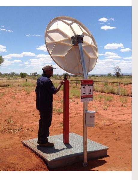
This solution works regardless of the user mobile device technology, and can be used in conjunction with any mobile network provider's network. In situations where a distant town provides multiple (Telstra, Optus, Vodafone) services, a single mobile phone hotspot can be used to connect with any of these services.
